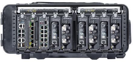
PacStar MRC is also available in PacStar Rack Mount Frame and other configurations ideal for ground vehicle and airframe mounted use cases including networking-on-the-move
